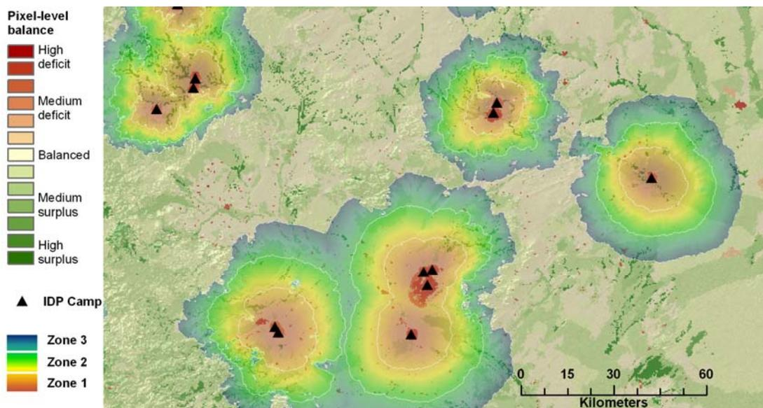
In the example shown the value assumed is 36 km on a flat accessible terrain or equivalent effort over rough and steep terrains. The supply/demand balance within these woodsheds and an estimation of the non-renewable fraction of the consumed woody biomass is given in Table 8.
